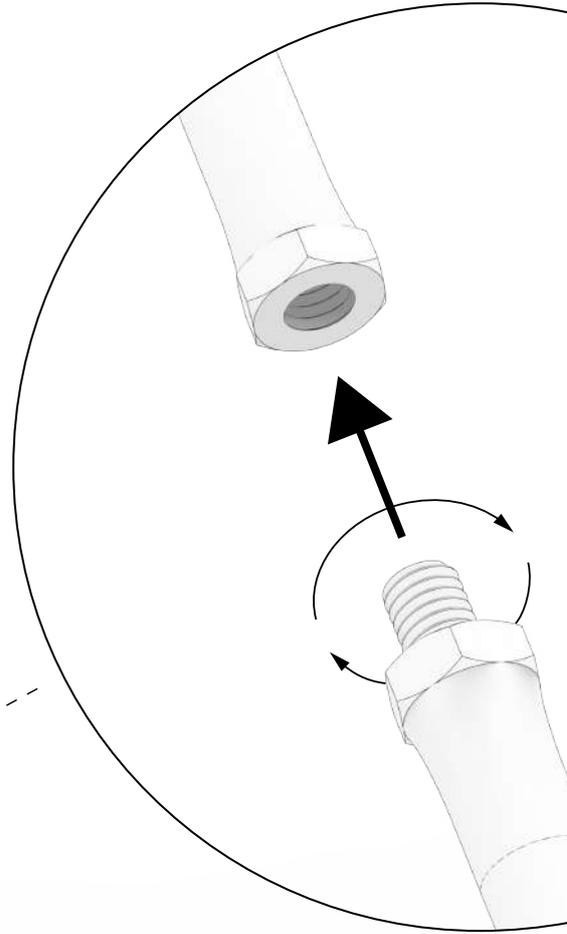
Each leg is divided in two sections. Screw them together, then screw the whole leg to the bottom of the disc plow.
