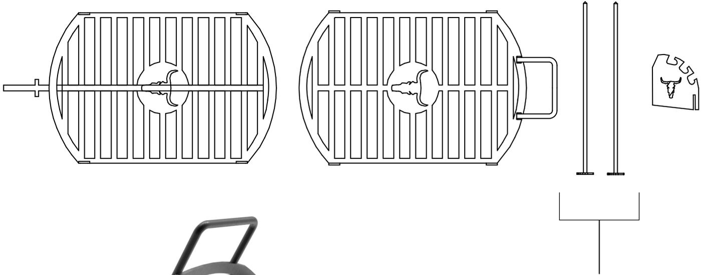
Use the fixing pins to secure both faces of the rack in the desired position
